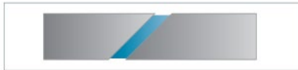
SCARF JOINT: A scarf joint is an angular butt joint. Cutting the joint at an angle increases the surface area.
