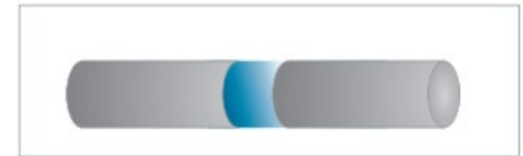
CYLINDRICAL JOINT: A cylindrical joint uses a butt joint to join two cylindrical objects.
