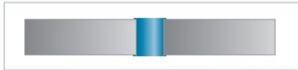
BUTT JOINT: A butt joint is formed by bonding two objects end to end.
