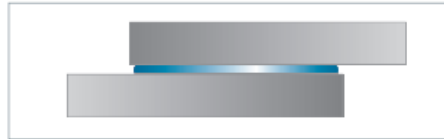
LAP/OVERLAP JOINT: A lap joint, also called an overlap joint, is formed by placing one substrate partially over another substrate.
