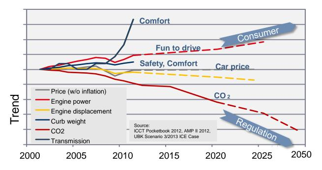
Powertrain Optimization and Innovation have to bridge diverging requirements: Long term CO<sub>2</sub> regulation vs increasing expectations of end customers
