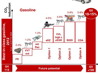
$\label{eq:VVT} \begin{tabular}{ll} VVT= \mbox{ variable valve timing } | \mbox{ SGDI} = \mbox{ lean burn } | \mbox{ FR} = \mbox{ friction reduction engine} \\ \begin{tabular}{ll} eDZ = \mbox{ extreme downsizing } | \mbox{ VVL} = \mbox{ variable valve lift } | \mbox{ high } \epsilon = \mbox{ high compression } \mbox{ cEGR} = \mbox{ cooled exhaust gas recirculation } | \mbox{ CDA} = \mbox{ cylinder deactivation} \\ \end{tabular}$
