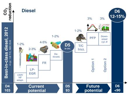
**CRP/HF**= common rail pressure / hydraulic flow | **LP-EGR**= low-pressure EGR system **FR** = friction reduction | De-Throttl. = de-throttling engine | **PFP**= low-peak firing pressure | **T/C** = turbocharger | **NSC** = NOx storage catalyst
