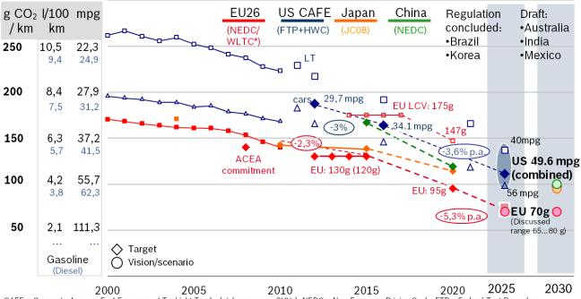
CAFE = Corporate Average Fuel Economy LT = Light Trucks (pick-ups, vans, SUVs) NEDC = New European Driving Cycle FTP = Federal Test Procedure HWC = Highway Cycle mpg = miles per gallon ACEA = Association des Constructeurs Européens d'Automobiles
